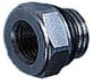
The Pulsoid inlet adaptor doubles as the retainer for the integral filter housing and an adaptor for the hose connection. Like the filter housing it is specifically designed and CNC machined from bright stainless steel, for durability and corrosion resistance.
