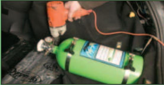
**1)** Mount the bottle to the boot floor, mark up the holes using a Tipex tip or something similar, then drill and mount the bottles using the supplied screws. (Make sure the bottle is mounted at an angle)
