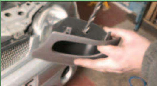
**9)** Decide on a suitable location for the arming switch and drill a hole to suit. We used the Wizards switch here for both kits, as it doesn't require a relay, meaning less wiring dilemmas for us - but the same applies for the Nytrex switch.
