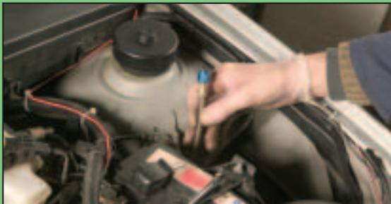
**3)** Feed the lines up and along the bulkhead to where the solenoids/pulsoids will be mounted. (It's a good idea to feed the electrical cable through at the same time if you're using a Wizards kit, to save time later).
