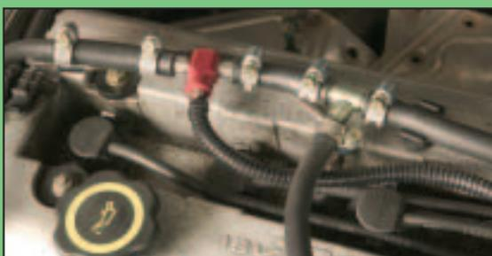
**6)** Find the fuel feed to the injectors and T into it with the supplied fuel connector. You may need to sleeve this tough plastic pipe as it's usually a pain to manipulate over the union ends.
