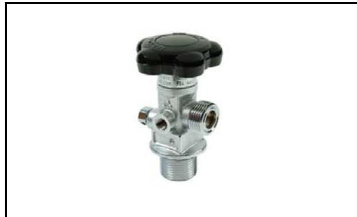
General pupose valve which was NOT designed specifically for nitrous use. Made from cast brass which is then chrome plated. Fitted with 6mm BRASS stem (which is easily broken rendeing the valve useless) and a very crude rupture disc for 'safety'. Has limited life span and weighs much more than a MaxFlow valve
